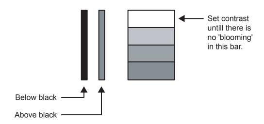
**CONTRAST** until there is no blooming (or distortion) in the brightest bar in the PLUGE pattern (see above). For Fixed-pixel displays, adjust contrast until there is a distinct definition between the two brightest bars.
